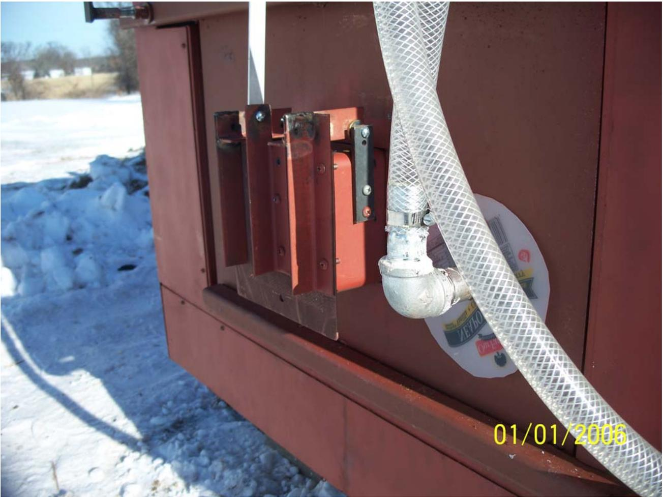
Place one of the damper hinge brackets to the side of the draft way, and mark the location of the holes. The bracket should be positioned approximately 3" back from the damper. Drill holes through the side of the draft way and then fasten the hinge bracket in position using screws or bolts. Repeat this process with the remaining hinge bracket.
