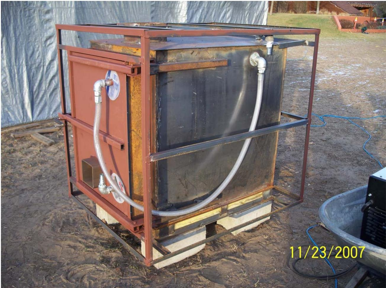
Install 1" hose barbs to upper fire door and water jacket elbows as shown. Install a length of 1" re-enforced vinyl hose between the door and stove inlet. Secure each end with hose clamps. Be sure to allow ample hose length so the door can open and close freely. Note: Submersing the end of the hose into hot water will soften it and make it easier to push onto the hose barb.
