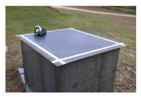
Orient the firebox so the front is skyward. Mark the fire door opening on the face of the front. The mark should be 1/2" inward on each side so a welding flange will be available after the door opening is cut. The author originally planned to use 2" wide masking tape to facilitate the marking but found a black magic marker to work the best.
